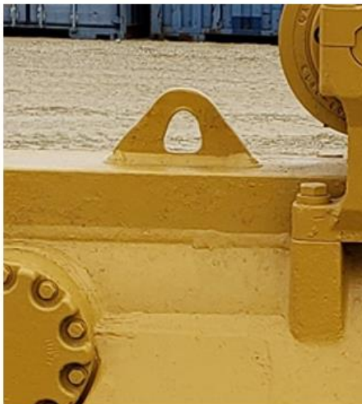
Example of a good lifting lug.
